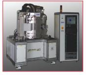
pilot to full production scalability. CFM is of "cold" deposition standards. It now allows single or multilayered film coatings onto sensitive polymer substrates or plastics which other deposition technologies would consider prohibitive. See www.applied-multilayers.com for coater and application data.
