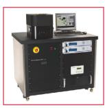
damage Plasma Enhanced Chemical Vapor Deposition (PECVD) plasma processing and Deep Reactive Ion Etch (DRIE). The system is based on a modular design starting with a universal chamber and cabinet unit with ICP etch and deposition bottom electrodes available for easy installation into the chamber unit. We are confi-
