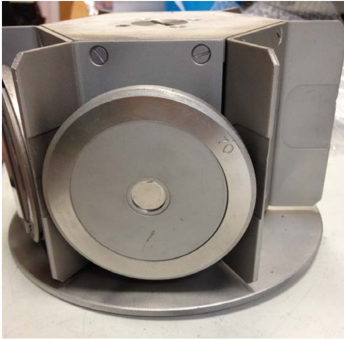
Fig 2 iButton sensor after NiCr coating
