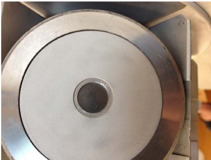
Fig 1 iButton sensor installed in substrate position on Plasma Coat substrate rotor
