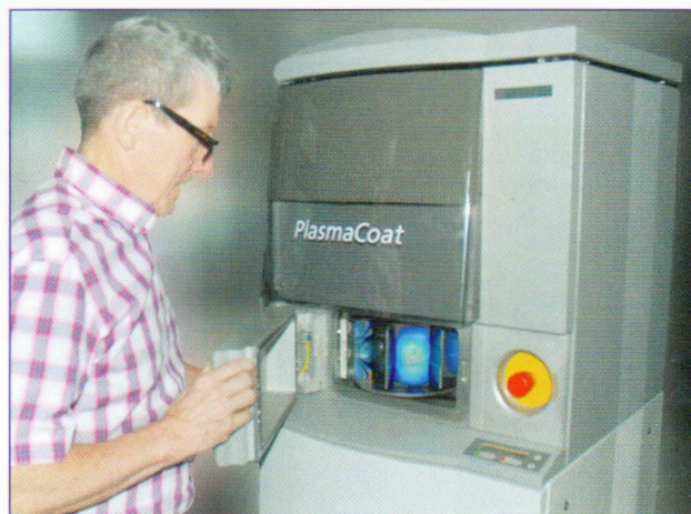
Substrate carousel mounted within loadlock with door open
