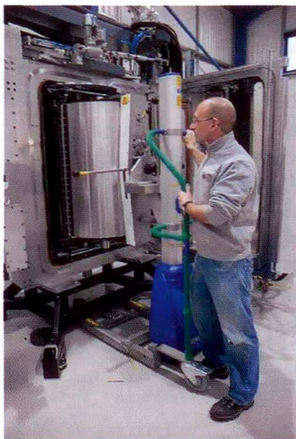
CFM1050 is equipped with 6 or 8 1.2m magnetrons.
