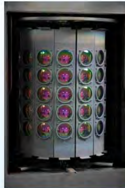
CFM650 used to apply mirror coatings to sunwear lenses in Shenzhen, China
